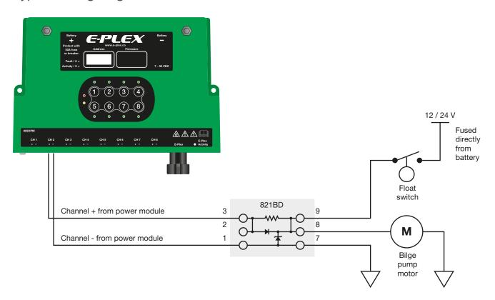
This example shows a single channel of the 821BD being used to power a bilge pump motor that is also supplied from a float switch.
