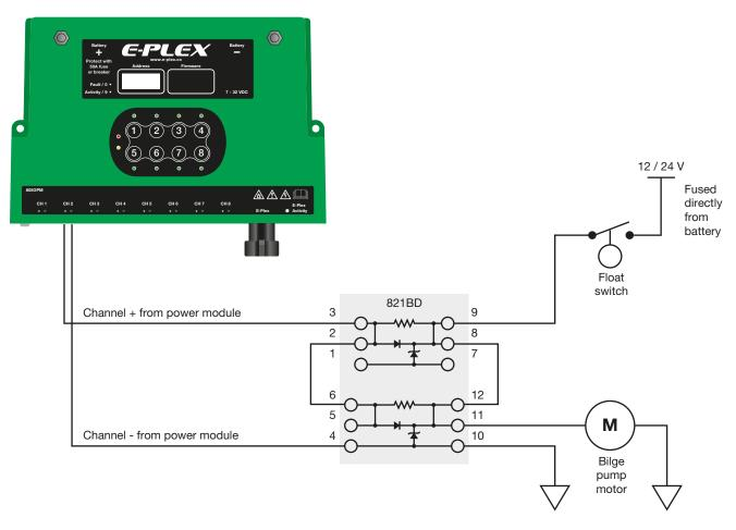
This example shows both channels of the 821BD paralleled together to supply an 8 A continuously rated bilge pump motor that is also supplied from a float switch.
